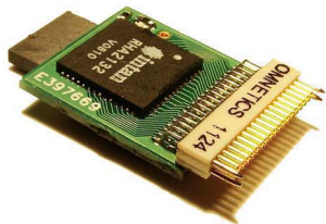
A 32-channel multiplexer
